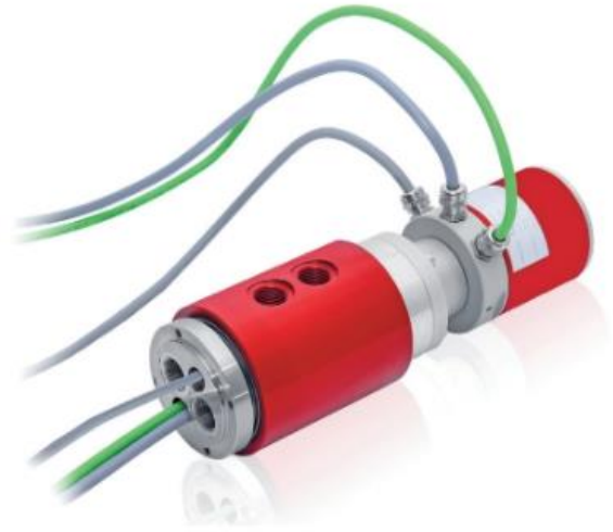
Fig. 3: KONSTANDIN designed and manufactured a total of 24 rotary feedthroughs for thyssenkrupp Automotive Body Solutions, each of which is equipped with two compressed air connections with G 1/2" threads, a signal cable for Profinet and two additional power conductors. Source: KONSTANDIN
